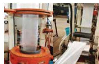
Manufacturing of bionanocomposite films using blown film extrusion
